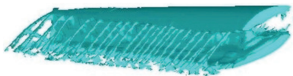
(b) Blade topology optimization result
