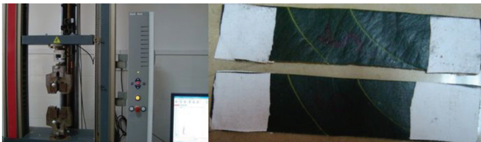
Fig. 10. The tension test of plant leaf
