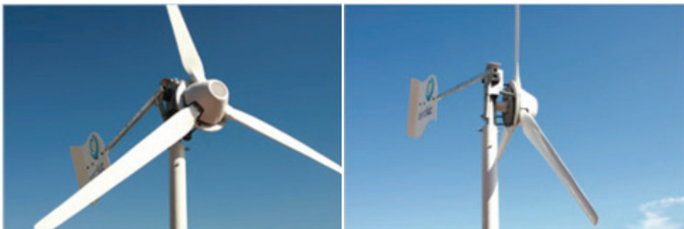
Fig. 9. Furling mechanism operating in a commercial wind turbine rated at 1.4kW. (a) Normal (unfurled) operation. (b) Furled turbine.
